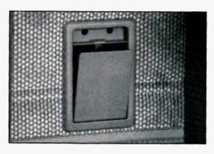
To remove the smaller ashtrays on each sidewall, press down on the tabs inside and pull out.
